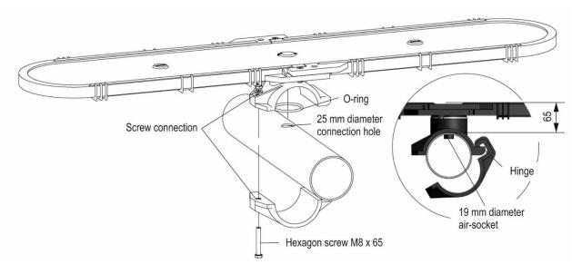
The hinge of the lower part of the clamp saddle is hooked into the upper part.
