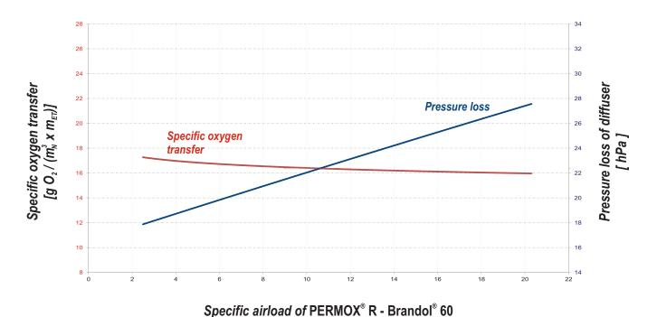
$[m_N^3/h \text{ per } m \text{ diffuser length }]$
