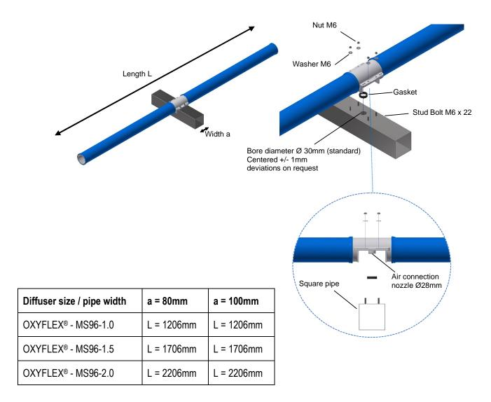
Possible pipe dimensions: Width: 80 mm or 100 mm (Further sizes are available on request)
