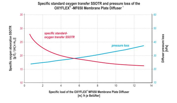
The values cannot be transferred to other plants. The results that are shown here depend on several influencing factors, such as the tank shape, blow-in depth, coverage or a separate recirculation due to additional mixers.
