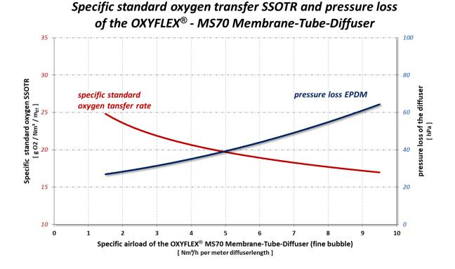
The values are not applicable for other waste water treatment plants! These shown results depend on several influencing factors, such as the tank shape, blow-in depth, coverage or a separate recirculation due to additional mixers.
