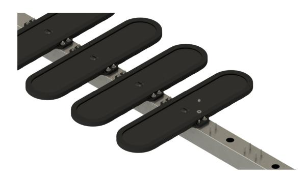
The OXYFLEX<sup>®</sup> - MF650 membrane plate diffuser consists of a flat, heavily ribbed base plate with air-sockets. A two-piece frame secures the membrane to the base plate. The base plate and the frame are made from fibre glass-reinforced polypropylene, and the membrane is available in EPDM or TPU.
