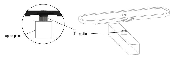
Screw connection between diffuser and socket must be sealed on site.
