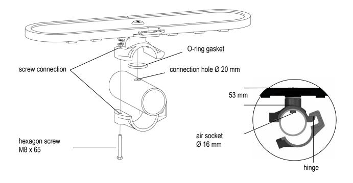
An O-ring made from EPDM is inserted between the upper part of the clamp saddle and the distribution pipe. The gasket between the diffuser and the pipe must be clean and undamaged.
