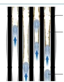
Polypropylene Filter Plate Bacteria, Viruses, Particles, Suspended Solids
