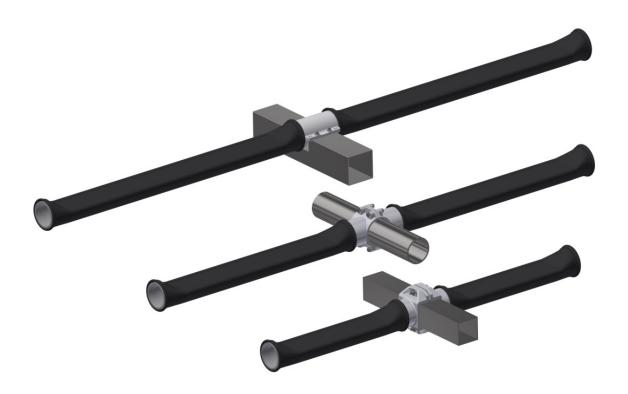
OXYFLEX® - OM Oval-Membrane-Tube-Diffuser type has a solid, strong oval tube body made of polypropylene (PP). The membranes are slipped over the body and each is fixed by two stainless steel 1-ear clamps (standard material AISI 304). The special oval shape of the body with the flat active membrane area results in a higher efficiency and significantly longer operation time in comparison to a normal tube diffuser.
