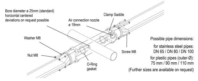
All Screwings must be tightend uniformily and crosswise in order to avoid tilting!
